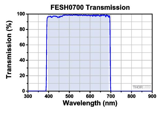
Figure 24 IR Blocking Filter Transmission Curve FESH0700
