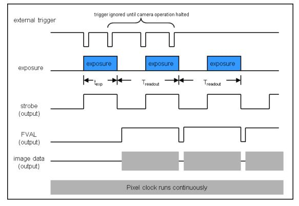
Figure 20 Timing Diagram – Standard, Frames per Trigger = 0 or > 1
