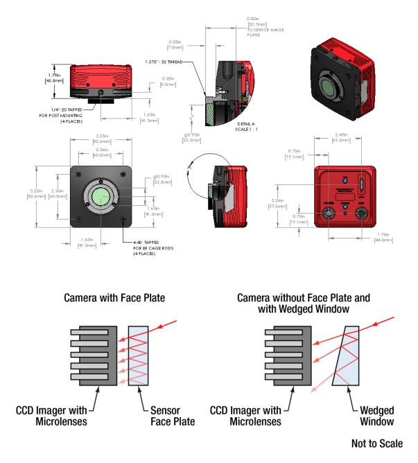
Figure 25 Schematic Showing Reduced Etalon Effects When Using a Wedged Window
