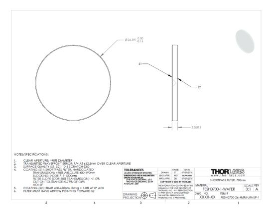
Figure 23 IR Blocking Filter Dimensions FESH0700
