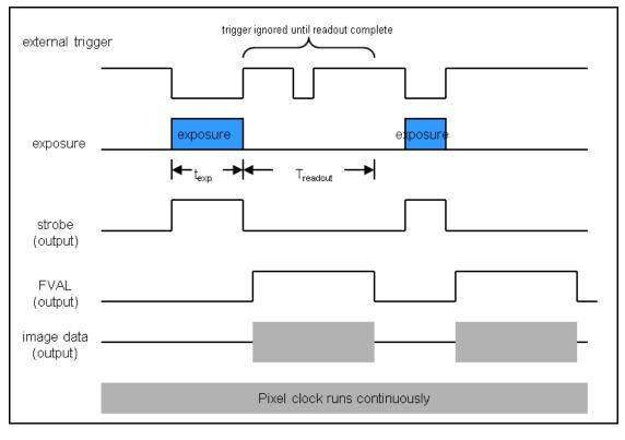
Figure 22 Timing Diagram – Bulb Mode
