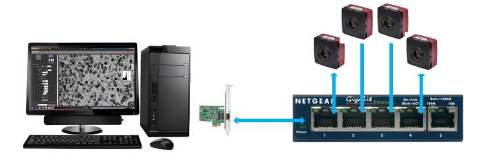
Figure 5 Gigabit Ethernet Switch Topology Setup for Multiple Cameras
