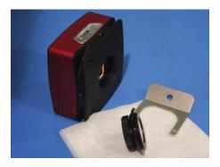
Figure 15 Loosening the C-mount and IR-Block Filter Assembly from Camera
