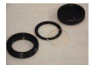
Figure 17 Removal of the IR-Blocking Filter from the Assembly
