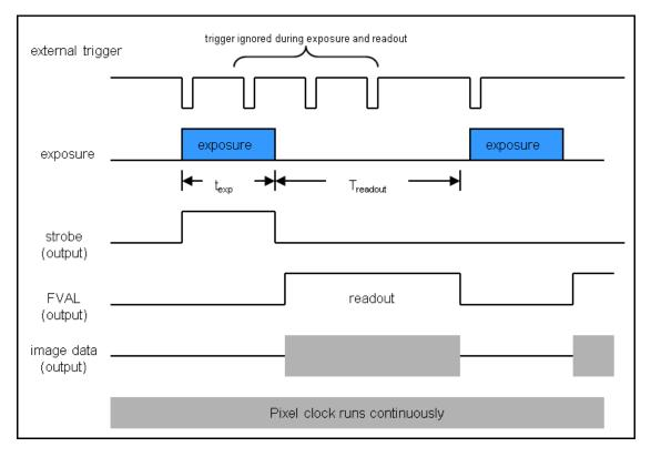
Figure 21 Timing Diagram – Standard, Frames per Trigger = 1
